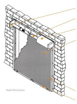
**BRACKETS** - Steel with powder coating to match curtain. Bolt to guide assembly and support counter-balance shaft and curtain.
